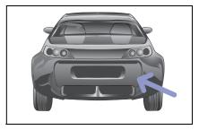
The rear fixing points are for towing other vehicles.
