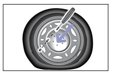
■ Screw the original valve insert (or the replacement one if necessary) back into the valve with the valve remover.
