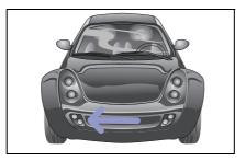
**Fixing points for the towing lug**The front fixing point is for towing the vehicle.
