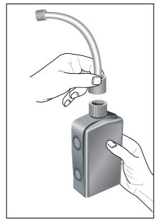
■ Screw the filler hose onto the bottle.
