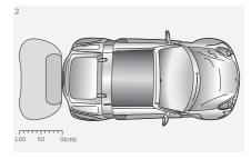
An obstacle is recognised from a distance of 100 cm behind the vehicle, at which time a beeping sound occurs. A continuous sound is emitted from a distance of 30 cm.
