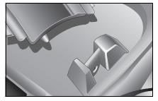
■ Guide the front end of the side rail into the mounting receptacle in the front luggage compartment.
