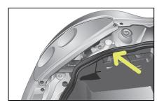
Topping up the windscreen washer system The windscreen washer reservoir has an approximate capacity of 3 litres. The headlight washer system\* also is supplied by the windscreen washer reservoir.
