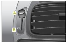
How to adjust the recirculated air or fresh air flow
