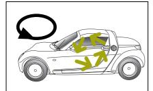
■ Select the lower position for recirculated air (B). The air circulates - e.g. when driving through a tunnel - in the passenger compartment.
