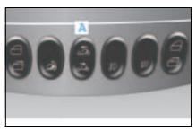
■ Press the rocker switch (A) in the "Open" direction.
