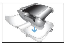
Inserting the hardtop in the hardtop bag\* for external storage  $% \left\{ \mathbf{n}_{1}^{\ast}\right\} =\mathbf{n}_{2}^{\ast}$
