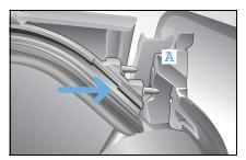
■ Guide the two side rail pins into the corresponding apertures (A).
