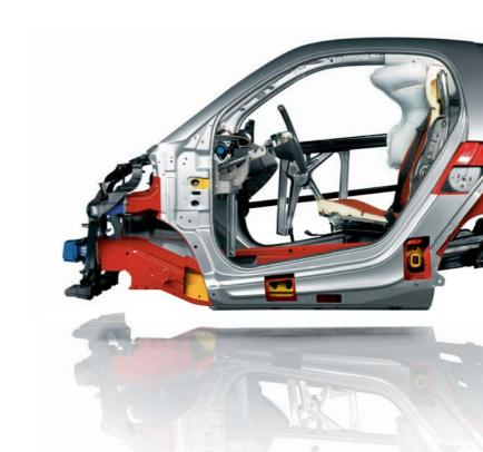
The tridion safety cell: additionally reinforced with high-strength steel sheets at strategically important points — for maximum stability, rigidity and strength.
