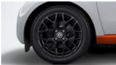
16" 8-Y-spoke alloy wheels painted in black, with front tyres: 185/50 R 16; rear tyres: 205/45 R 16
