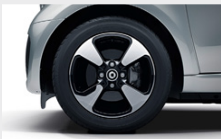
R32 15" alloy wheels in 4-spoke design painted black with high-sheen finish 165/65 R15 tyres on 5J x 15 ET32 (front), and 185/60 R15 on 5.5J x 15 ET42 (rear)
