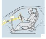
■ 2. In the event of a serious front-end collision, the steering column will retract telescopically out of harm's way.
