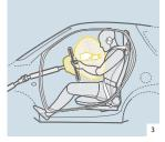
■3. All models are equipped with standard full-size front air bags and side air bags for enhanced protection from side impact.
