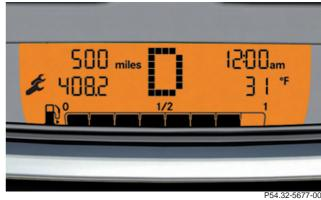
Multifunction display with maintenance interval display
