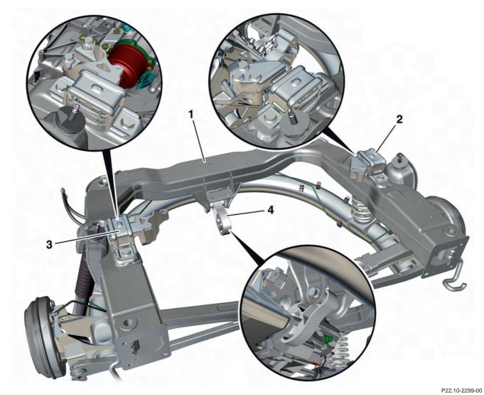
Engine mount, transmission mount and torque support
