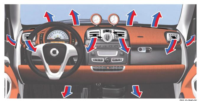
Air outlets for heater and temperature-regulated air conditioning
