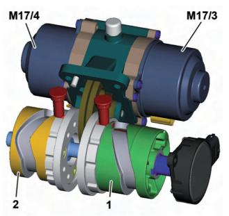
Transmission motor 1 selector drum Transmission motor 2 selector drum
