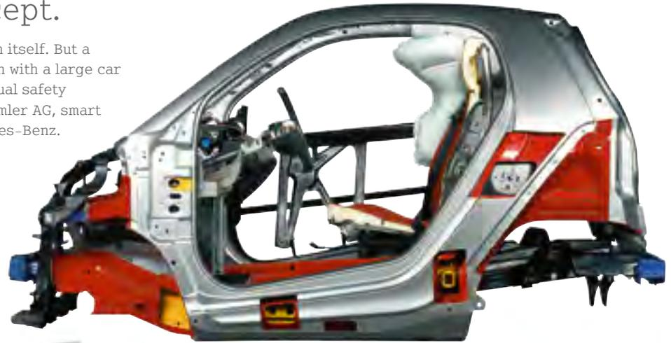
**The tridion safety cell:** additionally reinforced with high-strength steel sheets at strategically important points – for maximum stability, rigidity and strength. The impact energy is distributed evenly over the longitudinal and transverse members and so effectively reduced.
