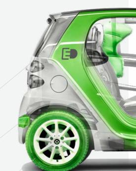
**Head/thorax side airbags:** the head/thorax side airbags that come as standard protect the head and chest in the event of a side-on impact. Additional safety is offered by the robust steel door structure.
