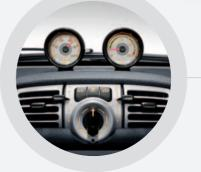
Dashboard instruments: show the battery stateof-charge and whether the vehicle is consuming energy or recuperating.
