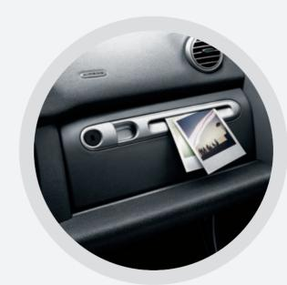
Glove compartment with clip function: with the practical clip function, you can keep notes, papers or photos within view at all times.
