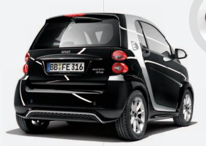
Charging socket: the charging socket is located on the right-hand side between the tridion safety cell and the rear lamps, behind the charging socket cap painted in the bodypanel colour. Its closing mechanism is regulated by the central locking function.
