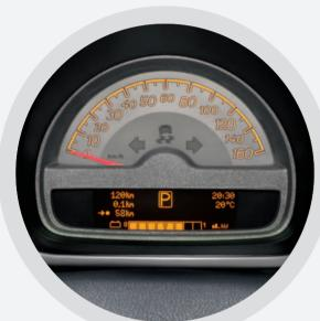
Instrument cluster with trip computer display: the multifunctional display has a READY indicator that shows when the vehicle is ready to go, an ECO display, a remaining range indicator, service interval indicator and settings for departure time and pre-entry climate control.
