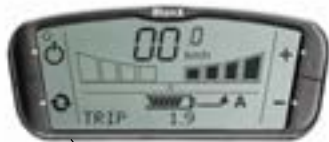
Drive mode – full power ahead: four bars in the basic display indicate the drive levels.
