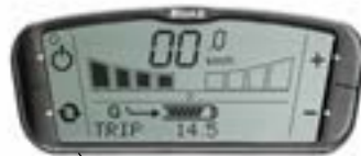
Generator mode – full energy back: four bars in the basic display indicate the generator levels.
