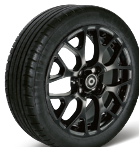
16-inch 8-Y-spoke alloy wheels (R95) painted in black, with front tyres: 185/50 R 16; rear tyres: 205/45 R 16
