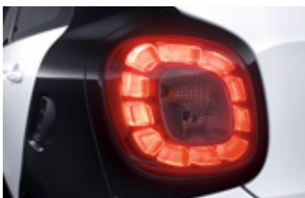
LED tail lights in semi-LED technology
