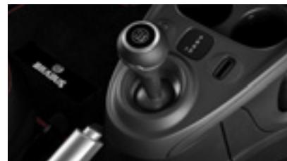
DCT gearshift lever [A453 277 0100]
