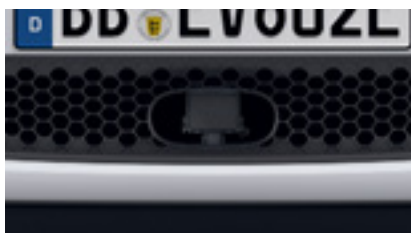
Radar sensor (Active Brake Assist)
