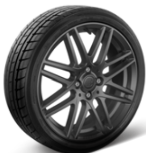
16/17-inch BRABUS Monoblock IX alloy wheels (R89) painted matt grey, with front tyres 185/50 R 16, rear tyres 205/40 R 17
