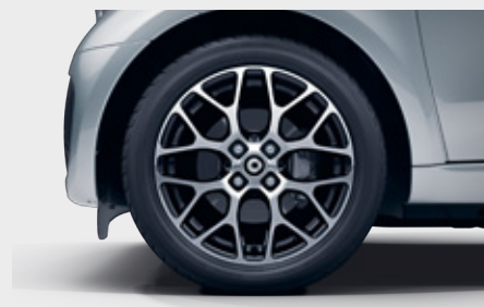
R56 16" alloy wheels in 8-Y-spoke design painted black with high-sheen finish 185/50 R16 tyres on 6J x 16 ET 44 (front), and 205/45 R16 on 6.5J x 16 ET 40 (rear)
