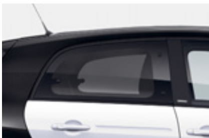
Heat-insulating dark tinted glass for rear side windows and rear window [E21]
