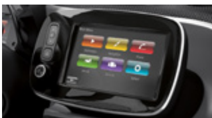
smart Media-System with 7-inch multi-touch TFT display
